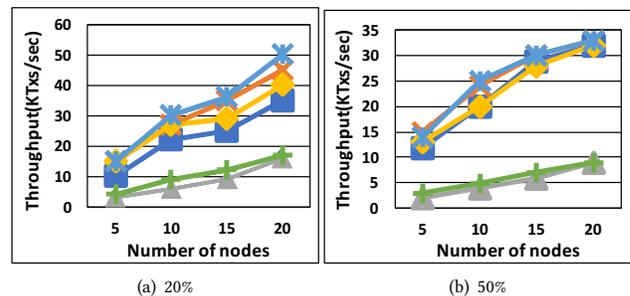
Figure 8: Throughput using TPC-C and by varying % of read-only transactions, the number of warehouses per node (W/n), and the number of nodes.
