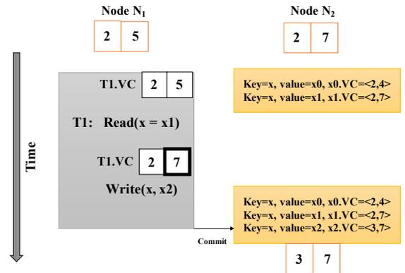
**Figure 4: Example of saving aborts due to reading fresher snapshots in update transactions. For the sake of simplicity, version-access-sets have been omitted. Update of  $T_1$ 's vector clock is shown in bold square.**
