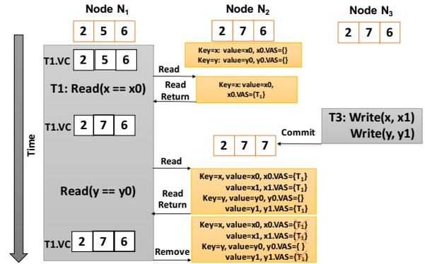
Figure 2: Example of execution where a read-only transaction advances its reading snapshot and still reads consistently. VAS is the version-access-set. Bold vector clock entries show where *hasRead* is true. The red crossed entries of VAS represent their elimination upon Remove.
